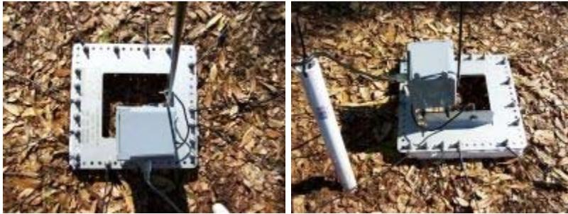
**Pictures Of The Coaxial Inverted L**
